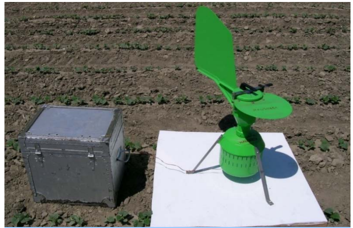
A spore trap used for monitoring airborne downy mildew spores.
