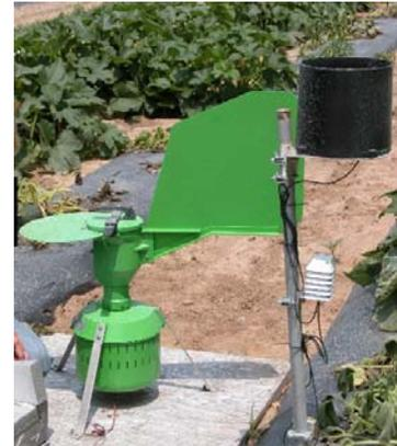
Figure 1. Spore trap in a cucurbit field.
